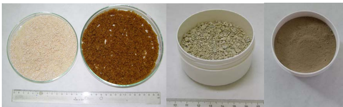
Fig. 1. Developed reference NORM materials: Ionex resin (water industry), sediment ( \text{TiO}_2 production), Tuff (building industry)
