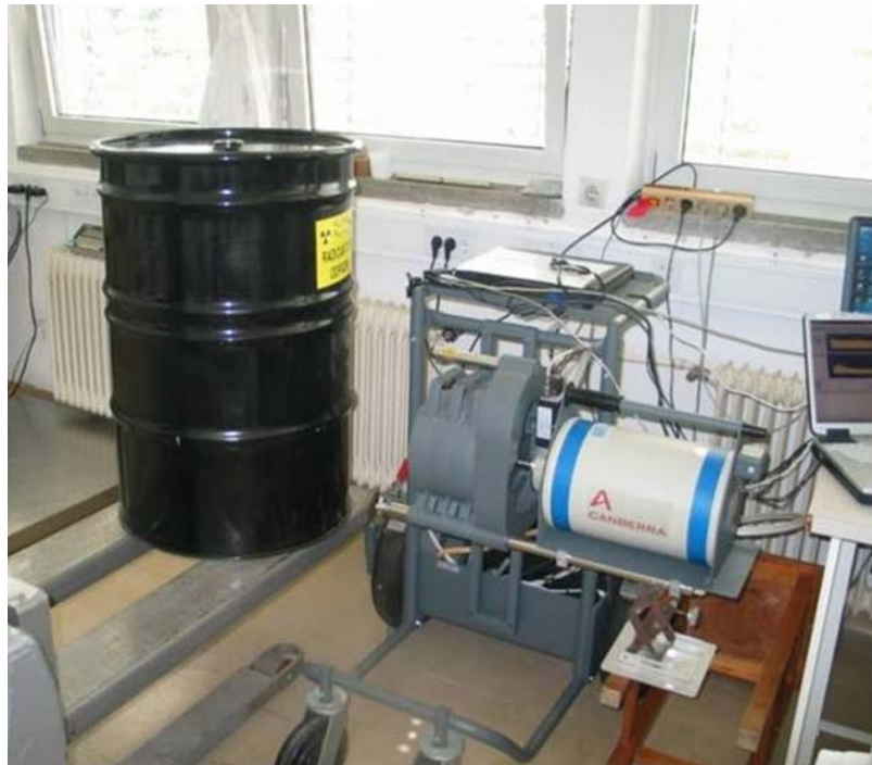
Fig. 10. NORM waste drum / gamma detector measurement configuration
