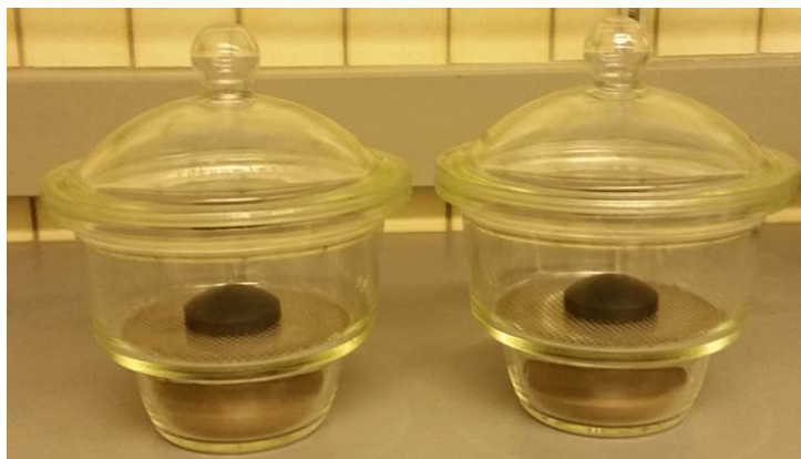
Fig. 12. Radon emanation measurement of building material samples
