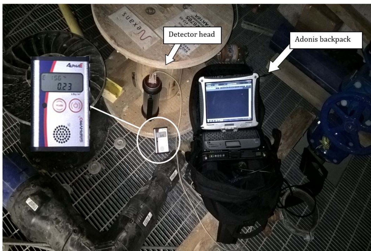
Fig. 3. The MetroNORM in-situ alpha-spectrometer system Adonis in operation
