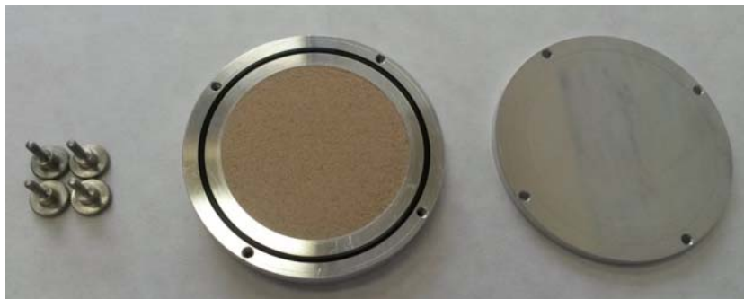
Fig. 2. Reference NORM sand source for use with the oil industry
