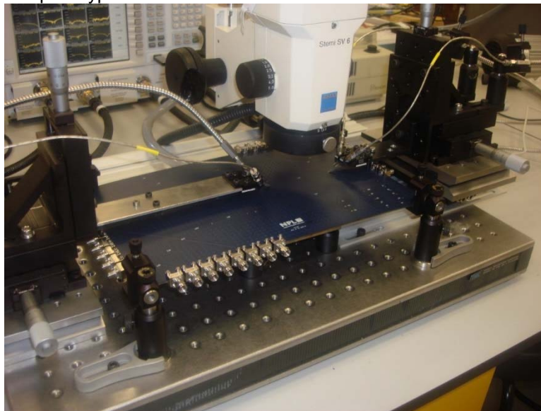
Fig. 11: Setup for measurement of mixed mode S-parameters showing the 4-port VNA, PCB probe station, GSSG probes and the prototype reference PCB under test
