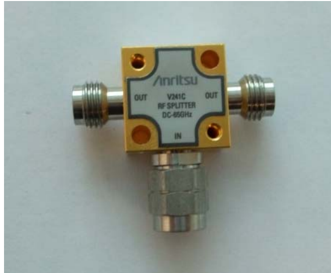
Fig. 7: Anritsu RF power splitter used as the device under test in an inter-laboratory comparison of multiport S-parameter measurements to 65 GHz
