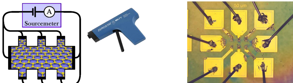
Fig. 9 Left: Carrier density tuning of graphene using a corona discharge device (the blue “gun”). The Hall bar resistance is monitored during the tuning procedure with a sourcemeter in voltage sourcing mode, using all the contacts of the Hall bar. Right: During the tuning procedure, the resistance of this device was monitored with a multimeter, using only the left and right contacts while the remaining contacts were left floating. The device was destroyed by a discharge through the graphene.
