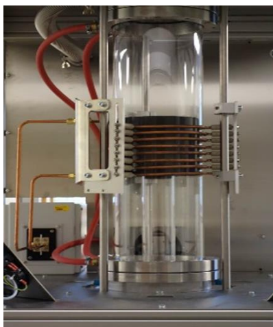
Fig. 1 Epitaxial graphene growth set up (left) and the growth crucible in a cross section
