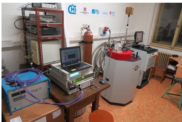
Fig. 35 A cryo-system, independent of external liquid Helium supply, with measurement equipment employed outside an NMI.
