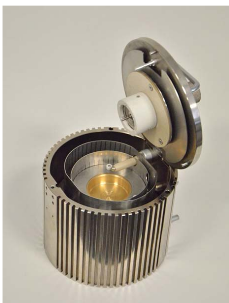
Figure 7 High temperature sample mount upgrade for aixACCT single-beam interferometer measurement system.
