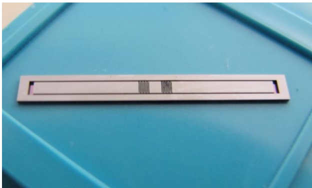
Fig. 4. Photo of the new silicon meander reference spring
