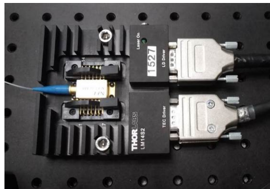
Figure 7. Left: Photograph of the vacuum system containing the optical cavity (two similar cavities in identical vacuum housings were manufactured with different finesses). Right: Lasers at different wavelengths were purchased for the detection of AMCs. In the photo is a 1527-nm laser mounted in a TEC cooling mount.
