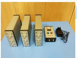
New Time Interval generators are stable enough (<3 ps) to be travelling standards for new Time Interval Supplementary Comparison in 2017
