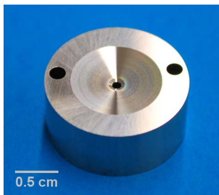
a) Cone standard from automotive industry provided by BOSCH
