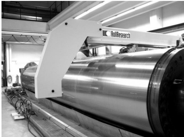
Figure 12: Four-point roller measuring device of a grinding machine
