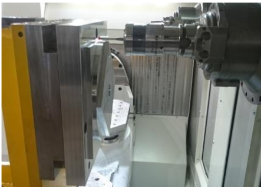
Figure 36: On-machine measurement of a workpiece replica
