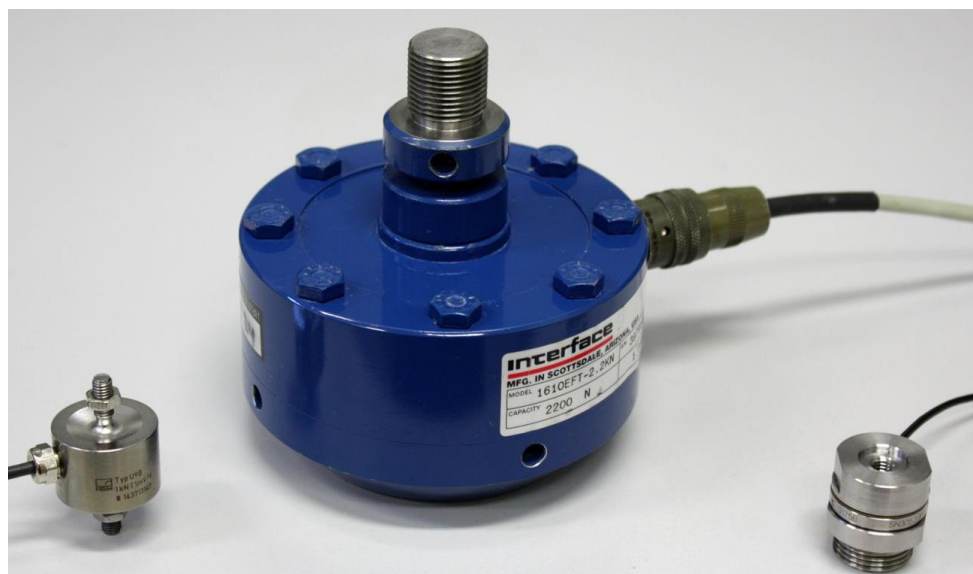
Figure 1: Set of force transducers selected for the investigations in all force calibration devices, HBM U9B (1 kN), Interface 1610 (2.2 kN), Kistler 9175B (-8 kN to 30 kN) (left to right).
