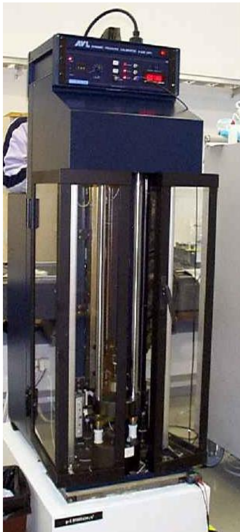
Figure 10: Drop weight devices at MIKES, with acceleration measurement of the drop mass either by accelerometer or by laser interferometer.
