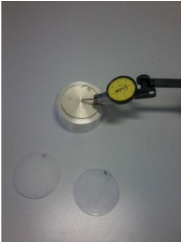
Figure 38: Series Cylindrical-shaped samples, and thickness measurement
