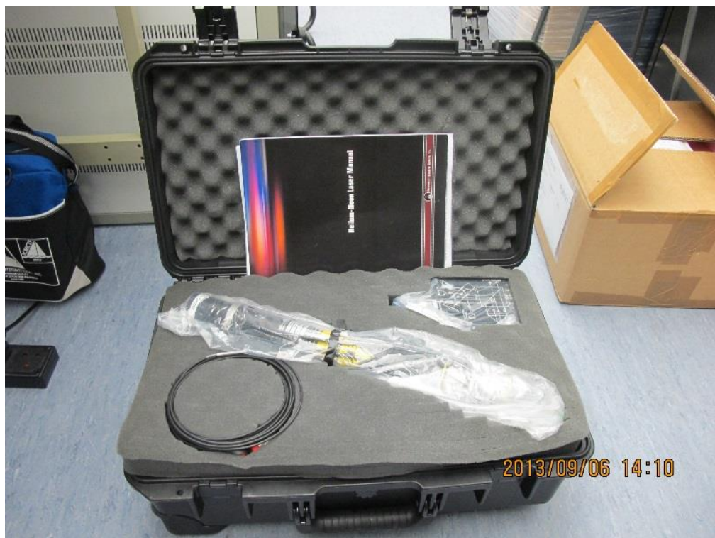
Figure 6 A portable Jamin interferometer system was developed at NPL.
