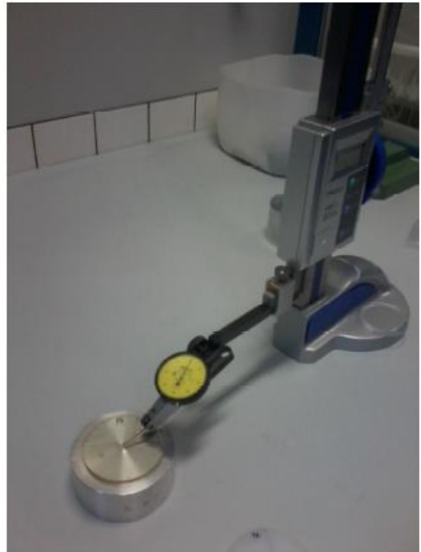
Figure 38: Series Cylindrical-shaped samples, and thickness measurement
