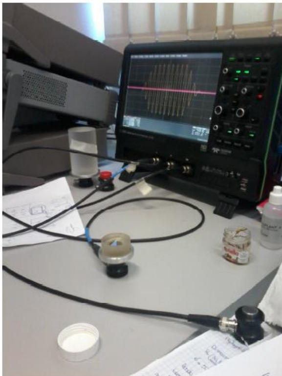
Figure 39: Preliminary tests of longitudinal and shear waves speed measurements.
