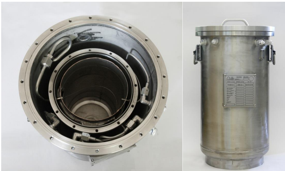
Figure 22: EDIE1 climatic chamber with and without covers
