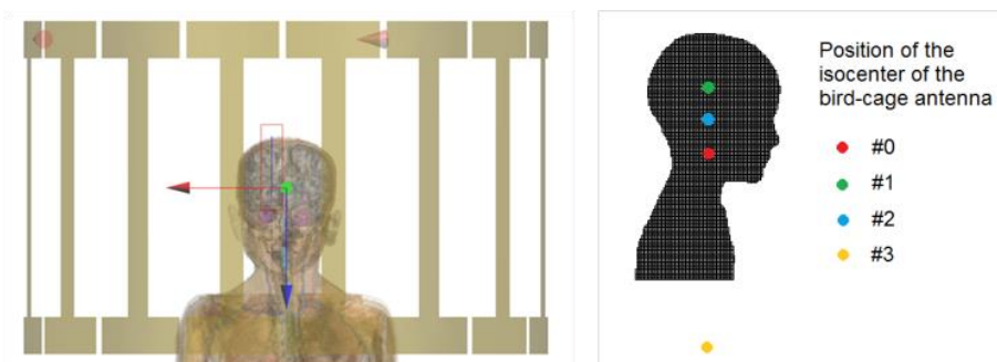
Fig. 3.6-6 (a) Roberta model with DBS electrode lead within birdcage coil used in FDTD simulations. The Huygens box is shown in red. (b) positions of birdcage coil isocentre relative to head used in simulations performed by INRIM.
