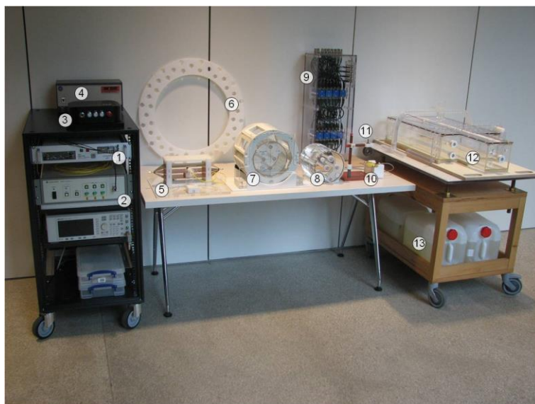
Fig. 3.1-1 Collection of components of the versatile measurement infrastructure for RF safety assessment: data acquisition system (1), OEFS-controller (2), H-TDS-controller (3), RF source and broadband PA (4), MR-TEM cell (5), annular gantry for body coil (6), head phantom in 8-channel pTx coil (7), second head phantom (8), 16 port Butler matrix (9), calibration coil (10) for RF current sensor (11), body phantom (12), phantom liquids (13).
