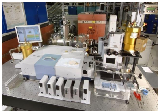
Fig. 3.2.8: FT-MLS: optical setup at the THz beam line of the Metrology Light Source.
