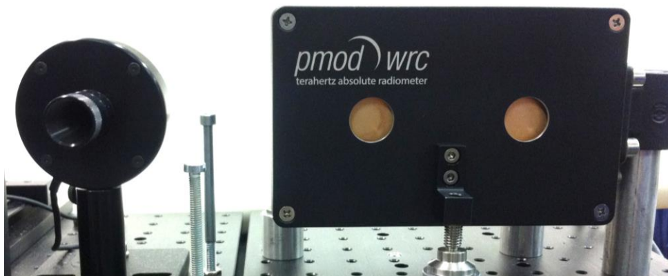
Fig. 3.1.3: The new PMO-THz radiometer (right side) together with the modified thermopile PTB THz-Standard-Detector.
