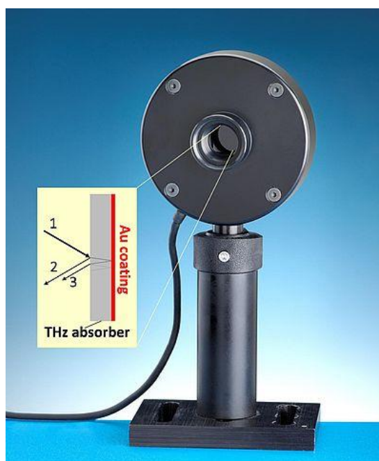
Fig. 3.1.1: PTB's new "gold standard" for detector-based THz radiometry: The cutaway view exhibits a schematic cross-section of the THz radiation absorber with gold (Au) coating on its back side. Part of the incoming (1) radiation is reflected (2) at the front side. The lack of interference modulation of this radiation indicates no remarkable residual (3) radiation after two passes through the absorbing disc enabled by the gold coating.
