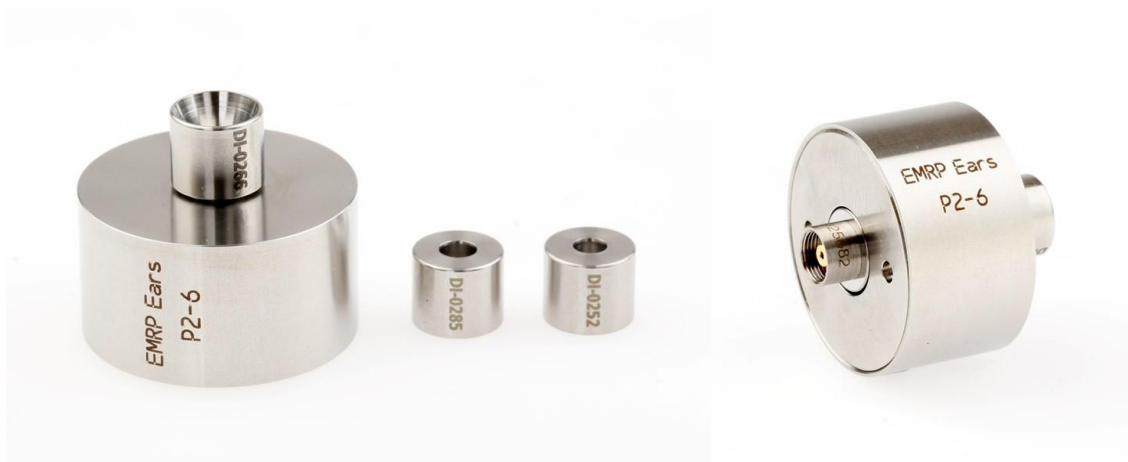
Figure 21: Photographs showing second prototype of neonatal ear simulator and adaptors
