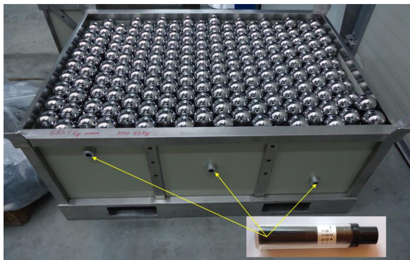
Figure 17: Metal phantom with Am-241 standard source
