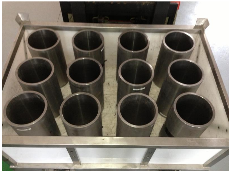
Figure 19: Steel tubes with Co-60 and Ag-110m in the measuring container
