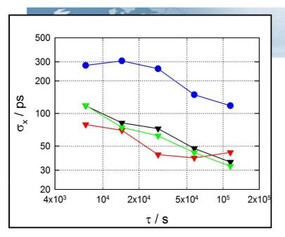
Time instability  $\sigma_x(\tau)$  of TWSTFT OP and PTB, (12/2011) analysis by OP; blue: standard operation of the network of 10 stations simultaneously
