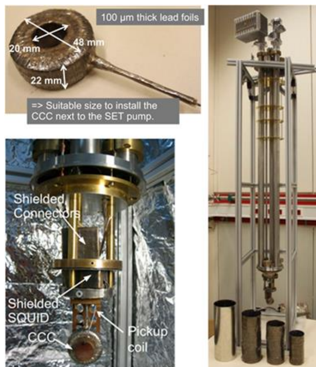
Figure 21: Elements of the 30 000:1 CCC current amplifier system developed within the JRP: CCC torus with lead shield (top left), installation of the CCC torus and SQUID (bottom left) in the dilution refrigerator (bottom right).
