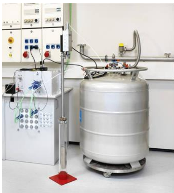
Figure 24: CCC resistance bridge setup at PTB (left side) and scheme of the calibration of an ULCA (input stage with a 3\text{-G}\Omega/3\text{-M}\Omega resistor network) with the 14-bit CCC (right side). From M. Götz et al., "Use of Binary CCCs for the Calibration of ULCA's", meeting of the TC-EM subcommittee "DC & Quantum Metrology" and Final Dissemination Meeting JRP Qu-Ampere, 27-29 May 2015, Bern (Switzerland).
