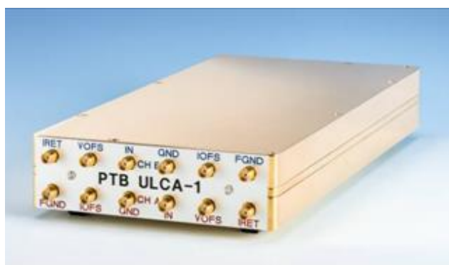
Figure 23: Left side: Photographs of a dual-channel ULCA prototype with copper housing and SMA connectors. Right side: Input current noise of two ULCA variants ( 3\text{ G}\Omega and 300\text{ M}\Omega total transresistance) in comparison with the noise of PTB's 14-bit CCC (input coil with 17 000 turns).
