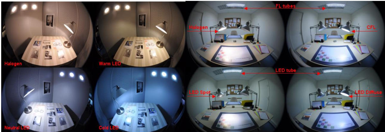
Fig. 3.21: views of four the identical compartments (left) and the four identical desks configuration (right) to assess visual comfort against the spectrum and the luminance distributions and the derived parameters (CCT, glare indices, gamut and colour rendition indices, light levels, light and distributions).
