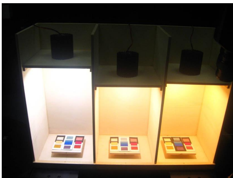
Fig. 3.22: Exposure boxes equipped with different white LEDs
