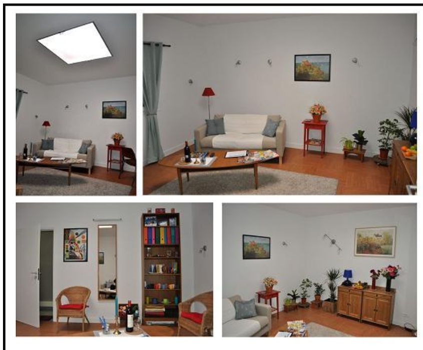
Fig. 3.19: views of the test room with the translucent diffusing panel in the ceiling. The room is furnished as a living room with many decorative objects of different materials and pigment, with real plants and a basket of real fruits/vegetables.
