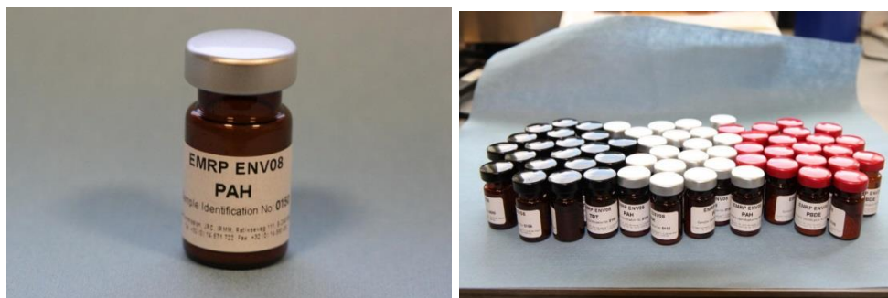
Figure 24: Model SPMs for PAHs (grey), TBT (black) and PBDEs (red) after jet-milling and filling in vials
