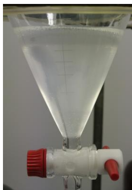
Figure 4: Extraction of PBDE congeners from HA containing water samples. Instead of a clear phase separation a kind of foaming can be observed. The foam has to be destroyed or prevented to successfully retrieve the PBDE.
