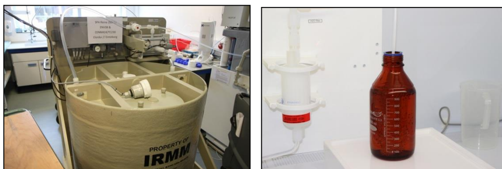
Figure 22: PFA-lined tank containing SPA mineral water (left) under constant recirculation while automatically filling bottles (right) by accurately recording the mass of water filled.
