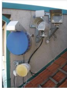
Figure 11: Left: the transmitter site of millimetre wave links, 58 GHz offset parabolic antenna, 93 GHz antenna. Right: example of observed rain attenuation event.
