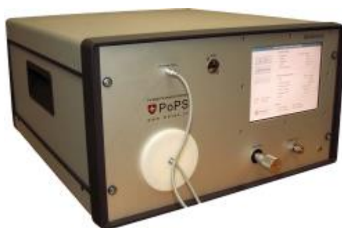
Figure 2: Representation of Traceable Mobile Permeation Generator (TMPG)
