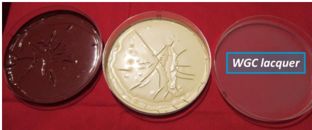
Figure 10: Comparison of the dry surfaces of a red matt, white matt and clear glossy lacquer
