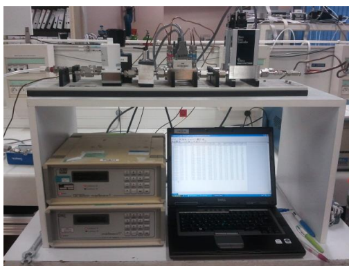
Figure 1: Representation of the Dynamic Dilution Standard (DDS)
