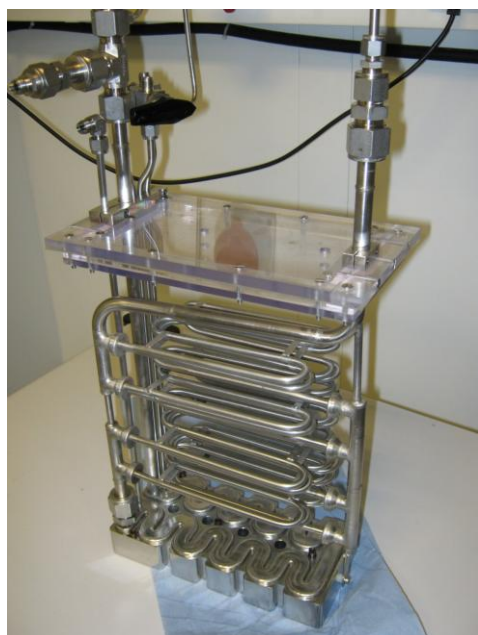
Figure 2. A photograph showing the saturator of the high pressure generator developed at VSL
