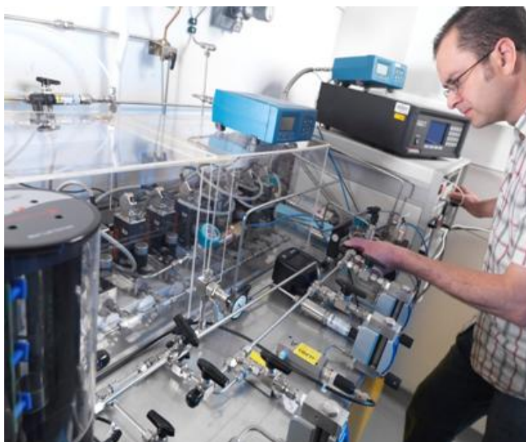
Figure 6. The facility developed at NPL for characterising humidity sensors with various gas mixtures
