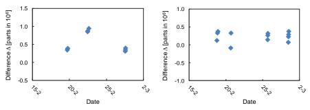
Example calibration results of a zero-flux DUT (LEM IT-600 S, ratio 1/1500, 0 - 600 A): small error, no significant different results for positive or negative currents, small effect of conductor position
