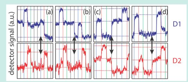
Error signatures of (a) P1 during sequential electron transfer, and errors by P1...P3 (b-d) during simultaneous electron transfer, showing "missing" cycles"
