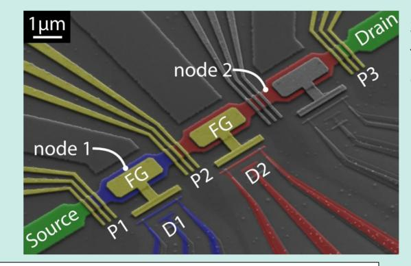
Self-referenced current source consisting of three pumps (P1...P3) serially connected via charge nodes, whose charge states are monitored by SET detectors D1 and D2
