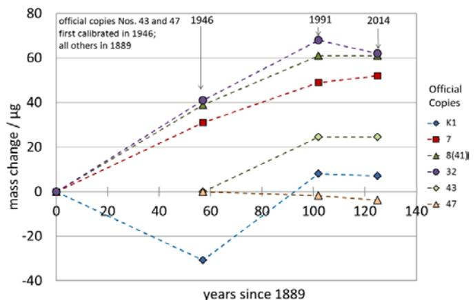
Figure 2: Fluctuations in mass differences between the International Prototype Kilogram and its copies
