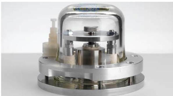
Figure 1: The UK’s copy of the International Prototype Kilogram (shown in protective casing)
