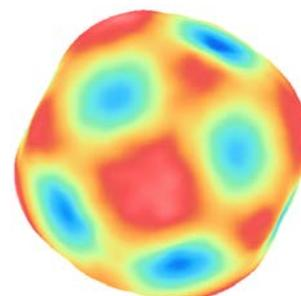
Figure 3: Topography of the AVO-28 S5 sphere showing a cuboctahedron profile
