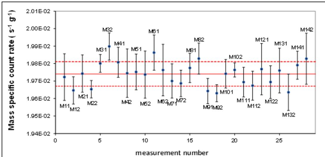
Figure 16 Homogeneity test measurements of the VUHZ cast steel samples used in the ILC\_1B exercise
