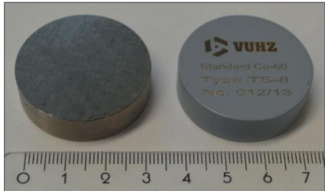
**Figure 3 above shows two of the cast steel reference sources produced in the project**
