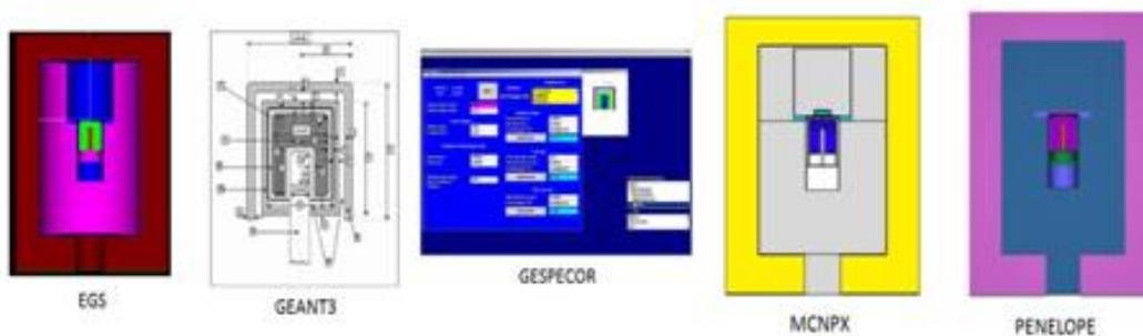
Figure 15 Graphical representation of the 5 Monte Carlo models of the Ge detector developed in this project. each one corresponding to a simulation package
