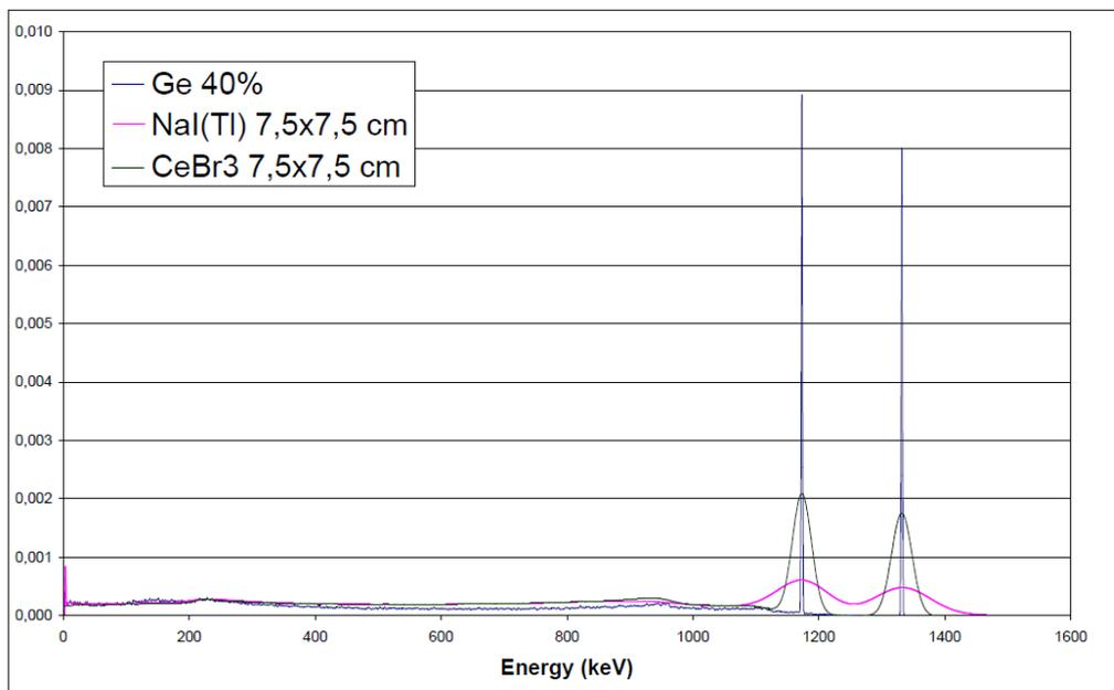
**Figure 1 Simulated gamma spectra of a source of Co-60 taken with three different detectors**
