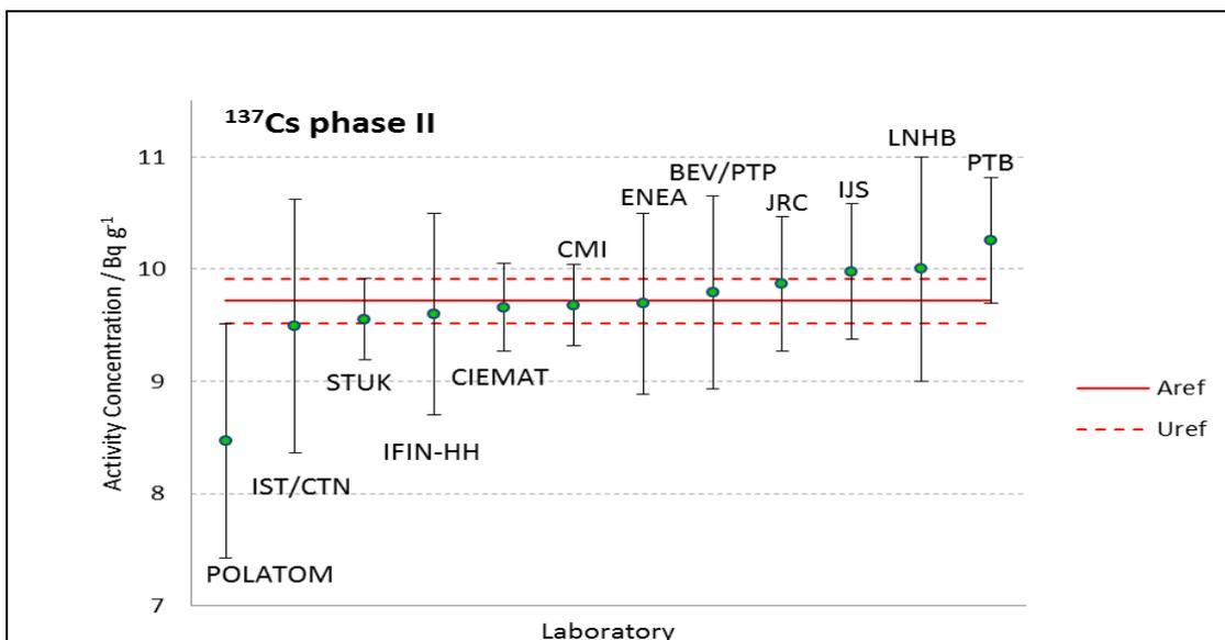
Figure 21 ILC-3 results reported for <sup>137</sup>Cs activity concentration in fume dust (ref. date 1 June 2013) in Phase II of ILC\_3. Error bars represent  $U_{lab}$ , calculated from the reported combined standard uncertainties, for  $k = 2$  and red lines the  $A_{ref} \pm U_{ref}$  ( $k = 2$ ). The consensus value  $A_{ref}$  is calculated from all reported values.
