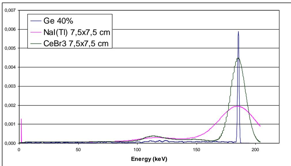
**Figure 2 Simulated spectra for a slag source containing <sup>226</sup>Ra measured with NaI, CeBr<sub>3</sub> and Ge detectors. Only the region corresponding to the gamma emission of 186.1 keV is shown**
