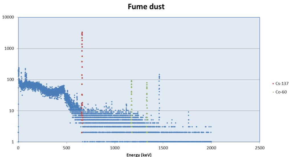
**Figure 13 Spectrum of fume dust sources contaminated with <sup>137</sup>Cs and <sup>60</sup>Co**
