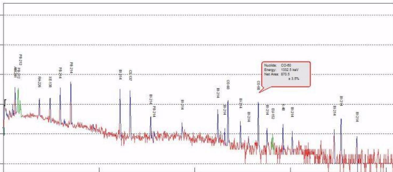
**Figure 25 Spectrum of a mixed source showing the identification performance of the HPGe-based prototype spectrometric devices**
