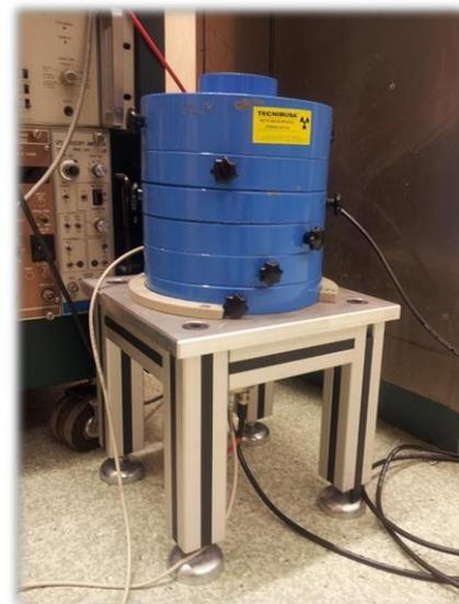
**Figure 26 Testing of a prototype based on a CeBr<sub>3</sub> detector at CIEMAT**
