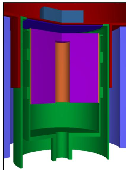
**Figure 22 a visual model of the CIEMAT prototype spectrometric device including a typical steel source**
