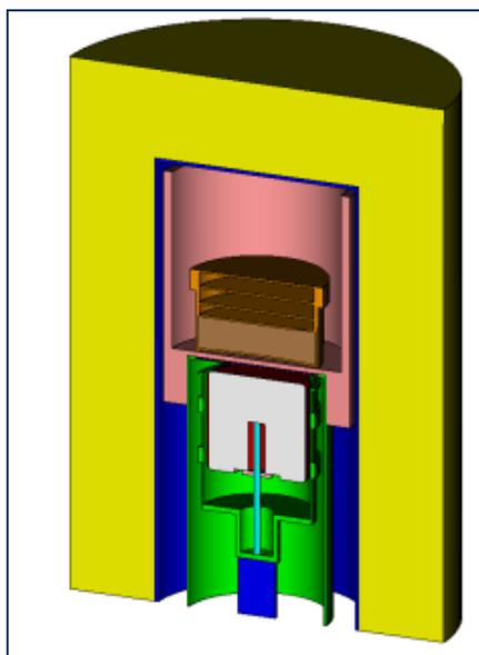
At PTB, a similar detector model was created using the MCNPX MC simulation package. Figure 23 shows a typical setup with a fume dust sample in a plastic container inside the measurement chamber of the prototype spectrometric device, on top of the Ge detector, whose relative efficiency was about 40 %
