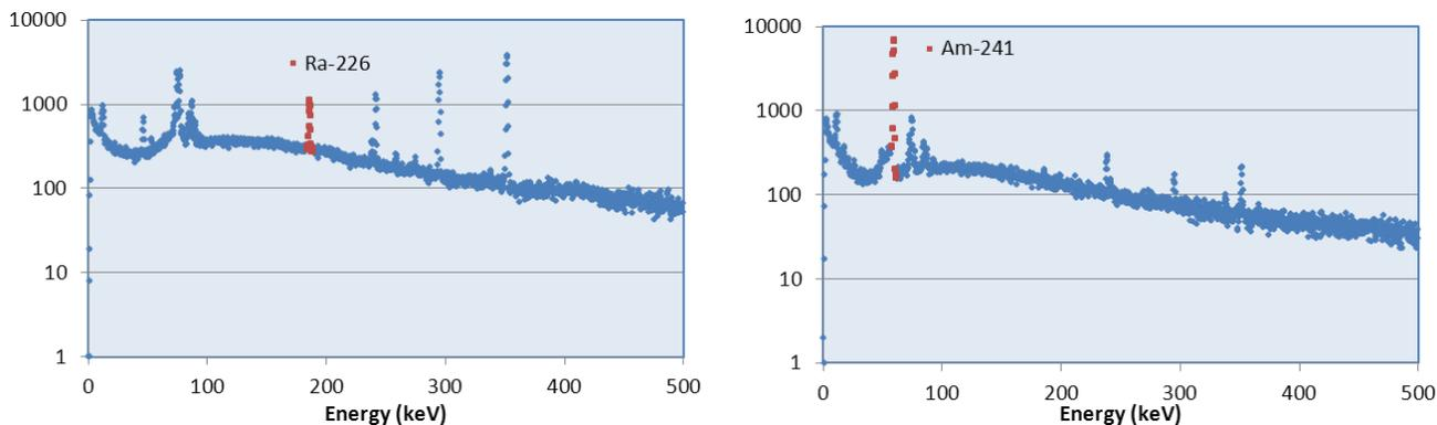
**Figure 11 Spectra of slag sources contaminated with <sup>226</sup>Ra and <sup>241</sup>Am**
