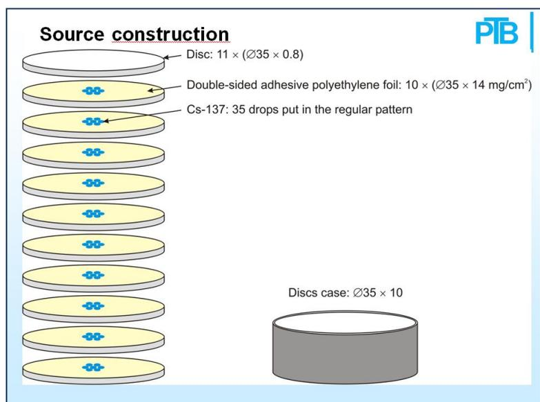
**Figure 5 Internal structure of composite steel sources**
