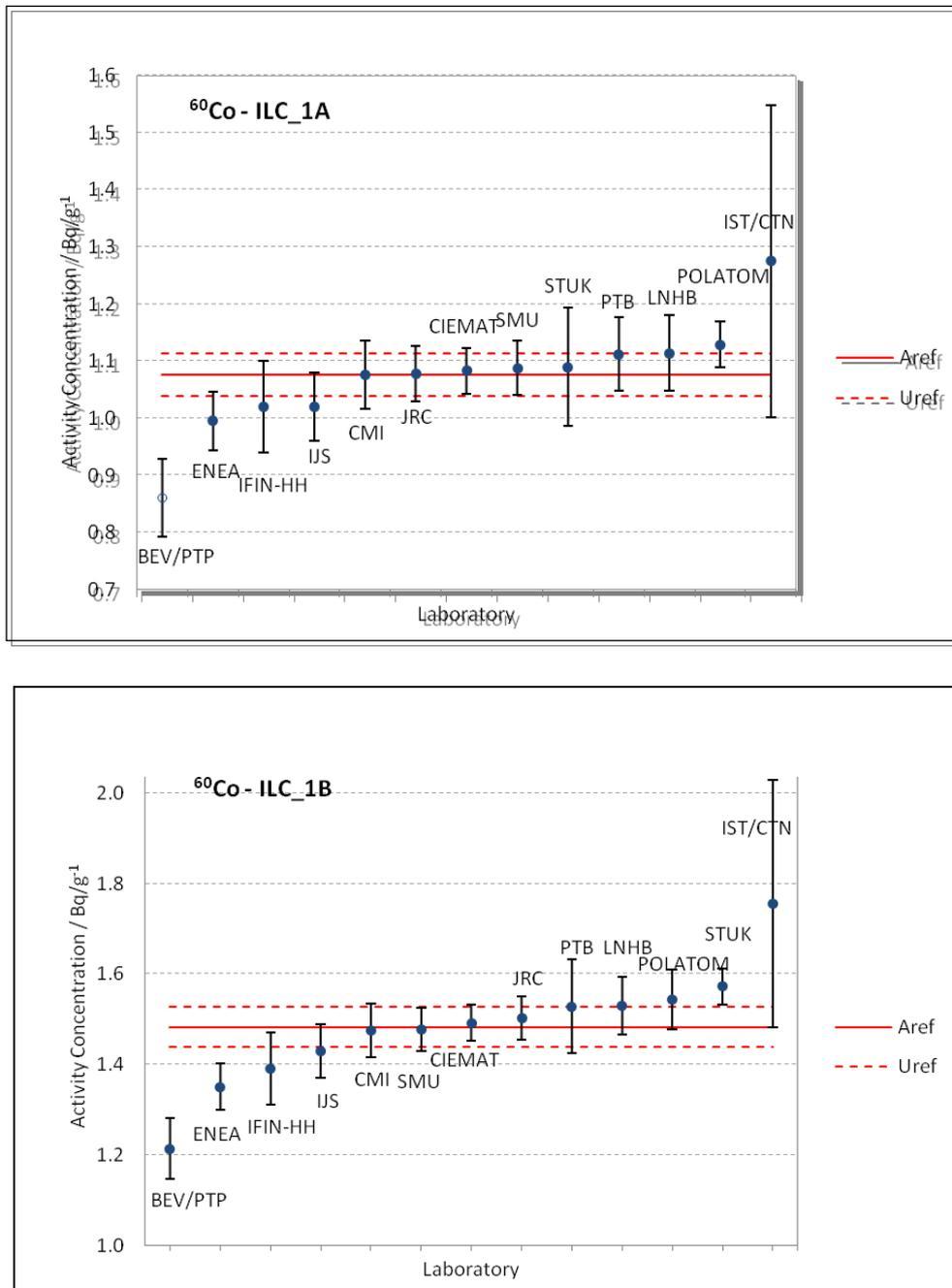
Figure 19 Laboratory results for <sup>60</sup>Co activity concentration in Siempelkamp and VUHZ cast steel samples. Error bars represent  $U_{lab}$ , calculated from the reported combined standard uncertainties, for  $k = 2$  and red lines the  $A_{ref} \pm U_{ref} (k = 2)$ .
