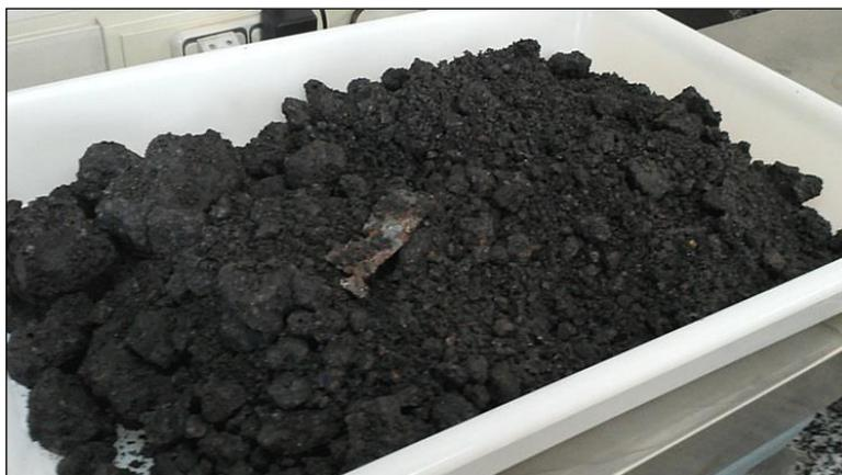
**Figure 10 Raw black slag from a steel mill factory used to prepare reference slag sources**
