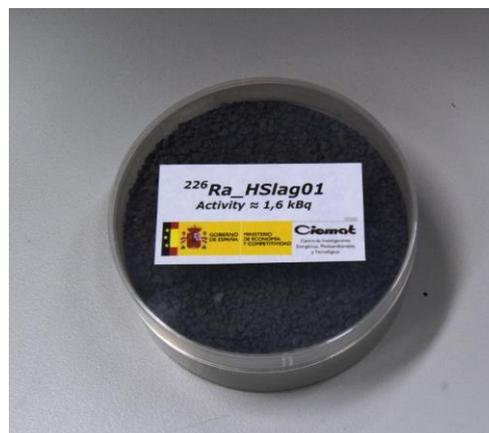
**Figure 9 Slag source contaminated with  $^{226}\text{Ra}$  in a cylindrical container**
