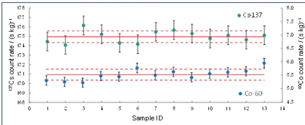
Figure 18 Homogeneity test measurements of the fume dust Cs-37 samples from the ILC\_3 exercise
