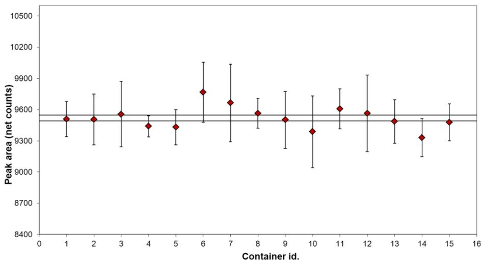
Figure 17 The mean net counts in the 186 keV peak of <sup>226</sup>Ra for each slag sample
