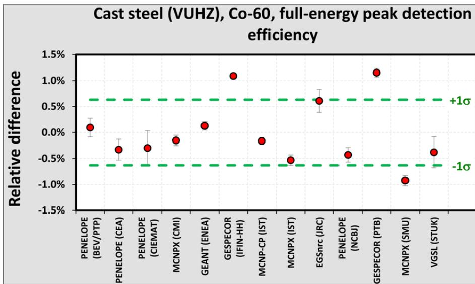
Figure 14 Results of the intercomparison of detection efficiency calculations with different Monte Carlo packages
