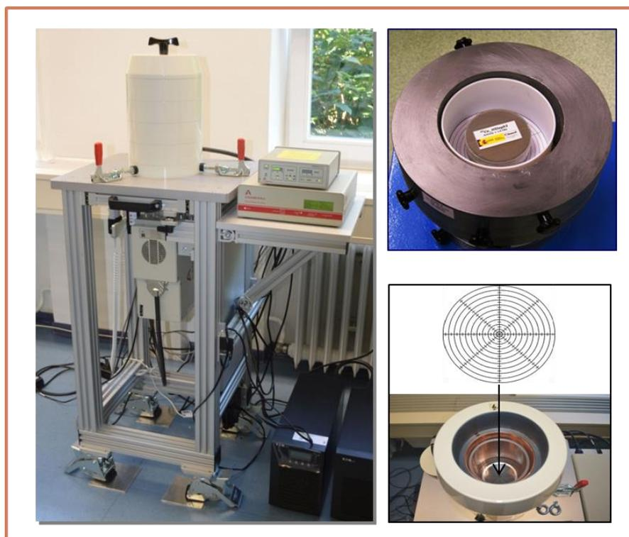
**Figure 24** The prototype spectrometric device built at PTB and the measurement chambers of the CIEMAT (upper) and PTB (lower) prototype spectrometric devices
