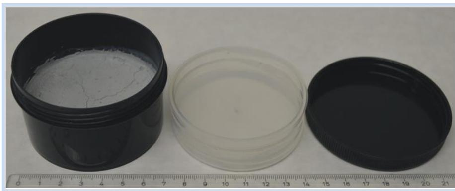
**Figure 12 Reference sources of fume dust produced in the project. Internal lids are used in the in the cylindrical container to keep dust under pressure and to maintain a reproducible geometry**
