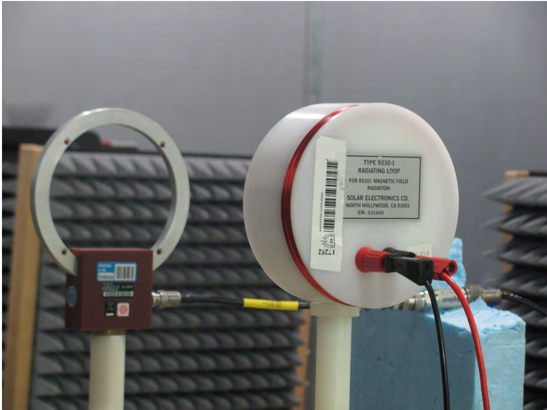
Figure 3. An example photograph taken during the calibration of the loop antenna for the frequency range 10 Hz – 100 kHz
