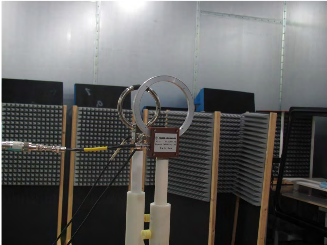
Figure 6. An example photograph taken during the calibration of loop antenna for the frequency range 2 MHz – 10 MHz
