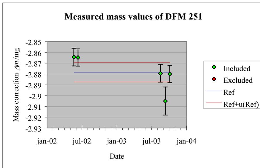
**Figure 1.** The results provided by the participants. The errors bars indicate the stated standard uncertainties ( $k=1$ ) associated with the results. The lines represent the reference values calculated from the results marked “Included” together with the associated standard uncertainty.
