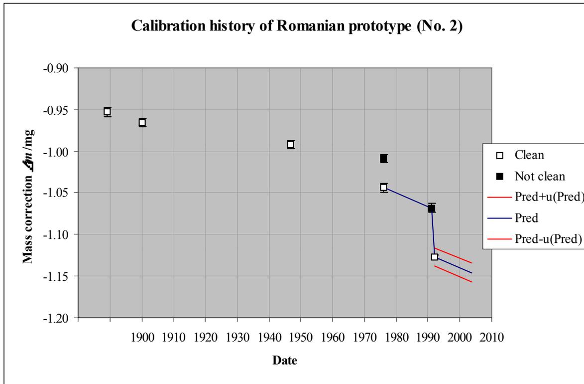
**Figure 5.** The calibration history of prototype no. 2. The full line “Pred” is shows how the mass of the prototype is assumed to have changed since the cleaning in 1976 and is used to predict the mass since the last cleaning and calibration in 1991-1992. The lines “Pred±u(Pred)” indicates the standard uncertainty of that prediction.
