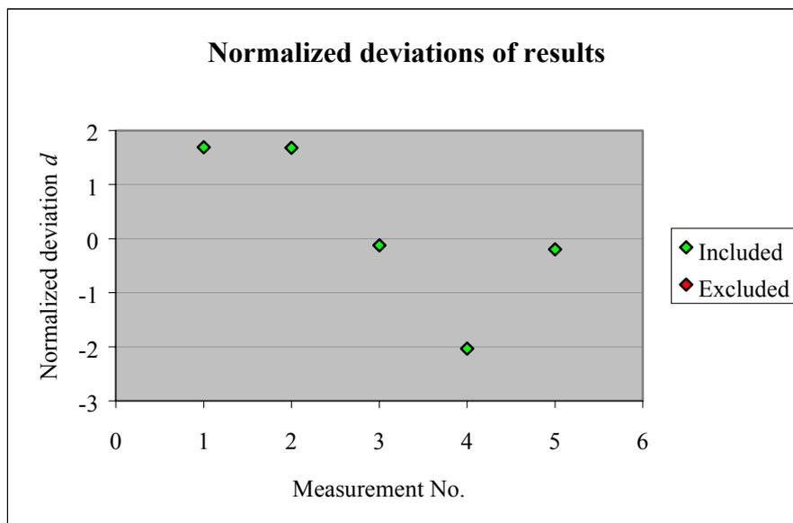
**Figure 2** The normalised deviations  $d$  of the results. Results with  $|d| > 2$  are classified as discrepant results.
