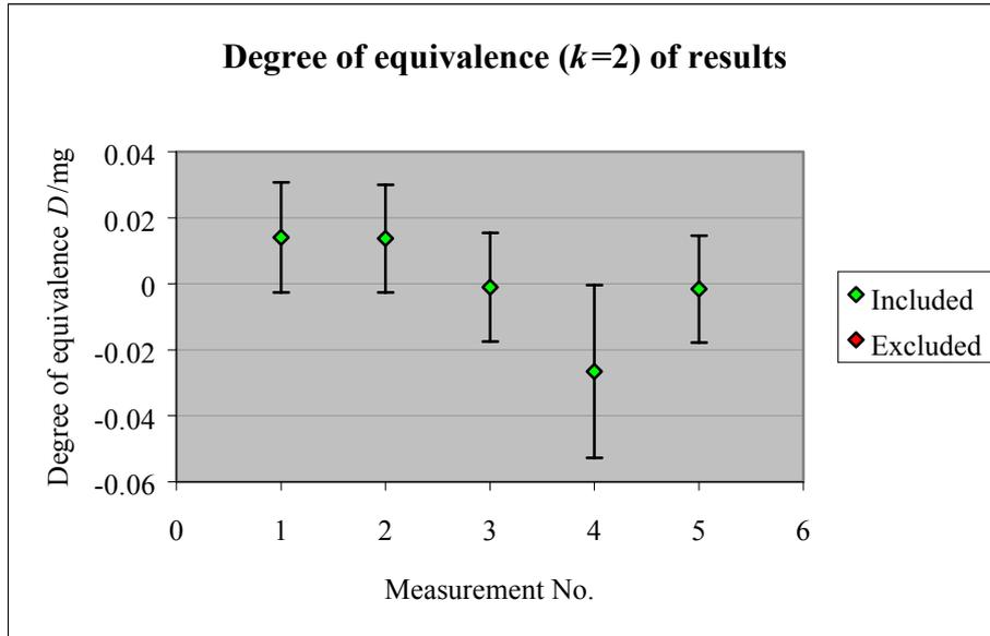
**Figure 3.** The degree of equivalence expressed as the deviation  $D = \Delta m - \Delta m_r$  and the expanded uncertainty ( $k = 2$ ) of that deviation.
