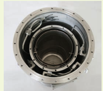
The MeteoMet automatic weather stations calibration chamber will be installed in the Everest Pyramid laboratory at 5050 m of altitude.
