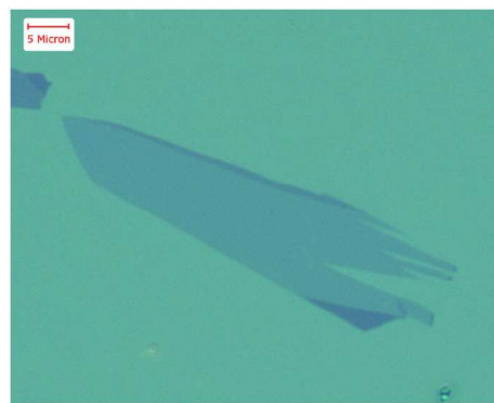
Fig. 1 Optical microscope image of a graphene single layer obtained by Scotch tape exfoliation from Highly Oriented Pyrolytic Graphite
