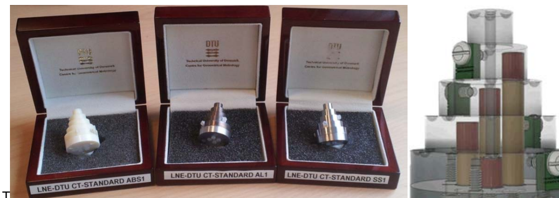
Figure 24: Three step cylinders in different materials and their internal structure.
