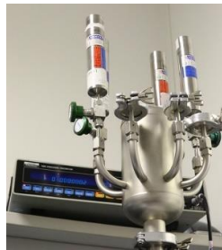
Figure 3 Reference leaks externally mounted on a leak detector (photograph courtesy of Vaseco Ltd.)
