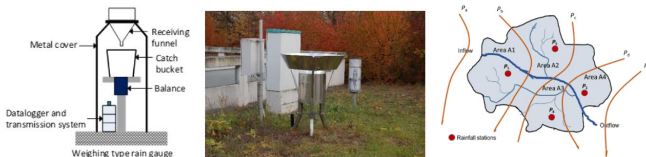
Figure 8 Schematic of weighing gauge (left), weighing gauge in the field (middle) and isohyetal method (right)
