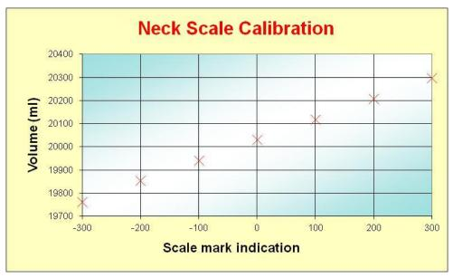
Figure 4. Neck scale calibration
