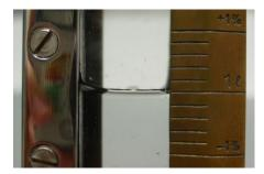
Figure 1. Standard test measure meniscus
