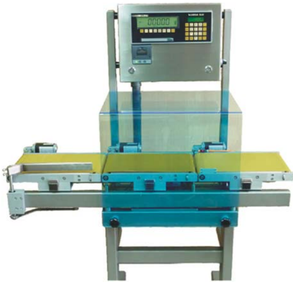
Figure 1. Automatic catchweighing instrument.
