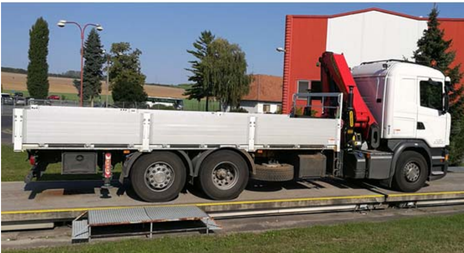
Figure 3. Automatic instrument for weighing road vehicles in motion.
