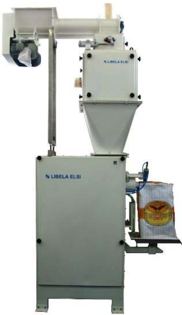
Figure 2. Automatic gravimetric filling instrument.
