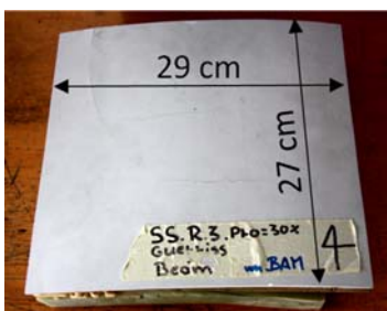
Figure 36: Schematic drawing of the cross-section of a wind turbine blade and images of section cut from a region near to the beams in the centre of the blade
