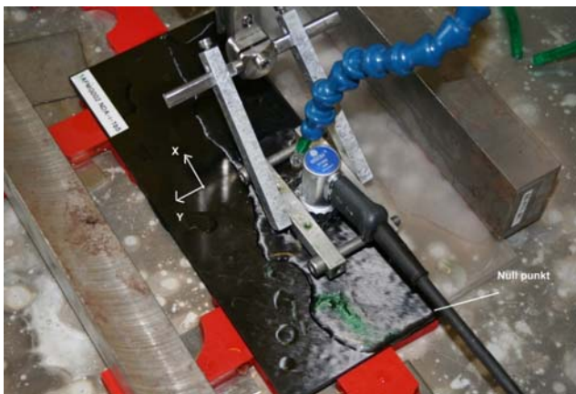
Figure 14: Ultrasonic phased array inspection set-up and manipulator (water coupled)
