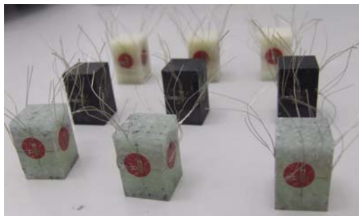
Figure 5: Strain-gauged out-of-plane compression samples, all lateral faces prepared identically.
