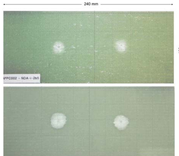
Figure 4: Example of 5 mm thick quadraxial NDA with 13 and 15J impacts showing evidence of surface indentation on the top face (upper) and extensive sub-surface damage zones on the rear face (lower).
