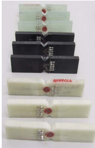
Figure 6: Notched and strain-gauged in and out-of-plane shear samples, front and back faces prepared identically.
