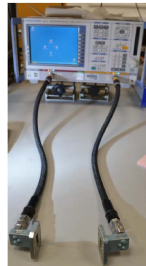
Figure 7: WG16 measurement cell, network analyser, flexible cables and waveguide transformers
