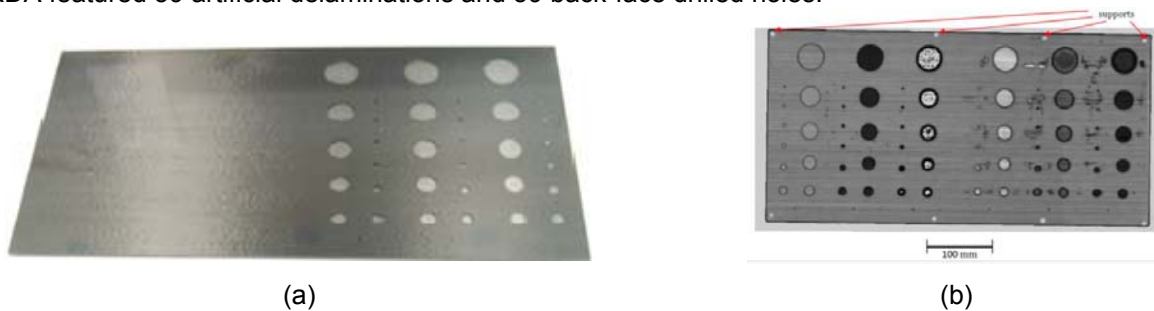
Figure 30: SE84 CFRP POD-RDA (a) back-face image and (b) ultrasonic C-scan (5 MHz, 3" focussed probe)
