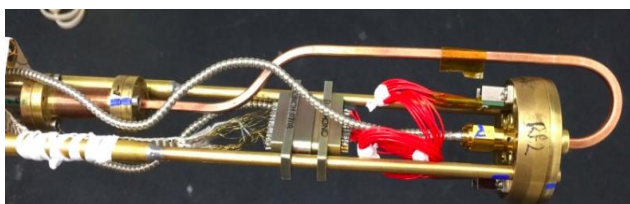
Figure 3.1.2.3. NPL's experimental setup for microwave photon detection using a semiconductor quantum dot. This shows a 180 GHz waveguide run from the top of the experimental probe to the sample holder (on the right), in which a quantum dot detector is mounted.
