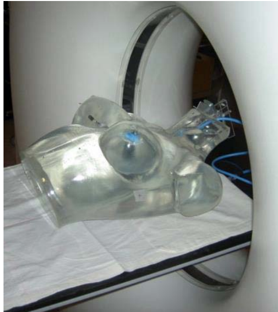
Figure 10: Anatomical female torso water phantom in which different type of chamber and heterogeneities can be set.
