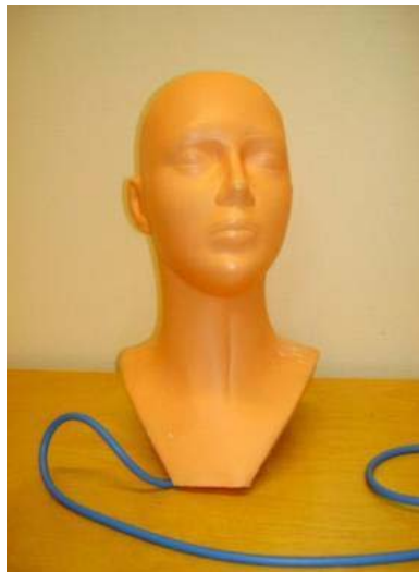
Figure 11: Anatomical head and neck water phantom with polyethylene wall 1 mm thick in which PTW semiflex chamber can be inserted in fixed position.
