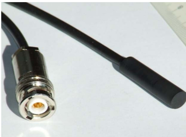
Figure 8: prototype of the Tor vergata/ENEA diamond based dosemeter
