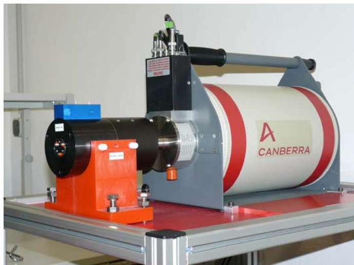
Figure 7: PTB Ge spectrometer assembly
