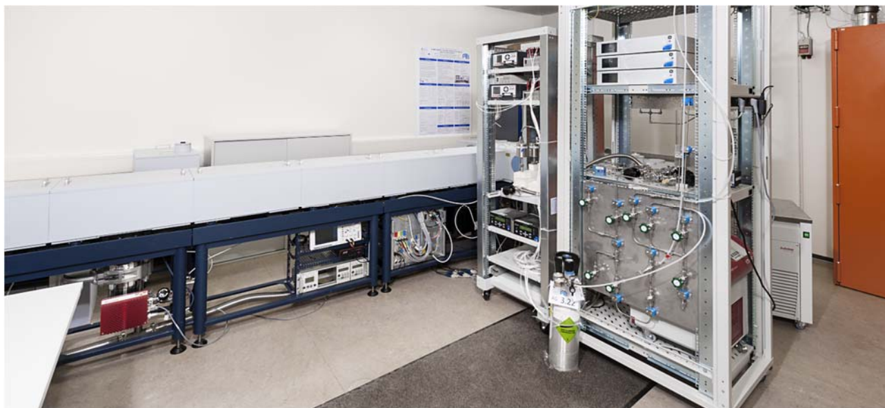
Fig. 1: Central facility Bruker IFS 125HR FTIR-spectrometer, gas manifold and continuous pressure and temperature monitoring setup.
