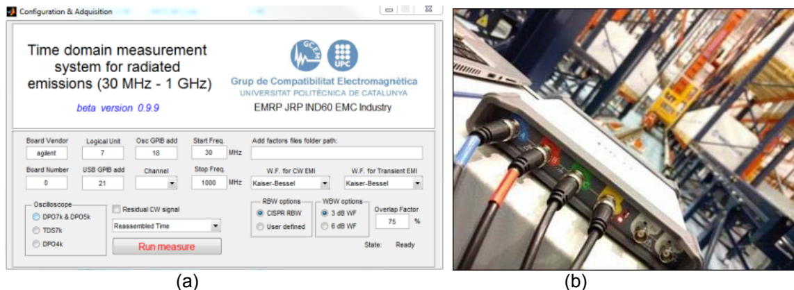
Fig. 25. Time domain radiated emission method (a) software, (b) measurement with pico-scope
