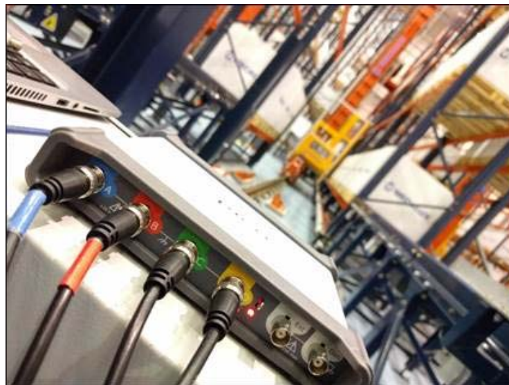
Fig. 8. A Time-Domain EMI measurement system.
