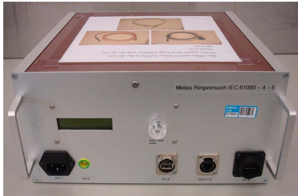
.Fig. 35. Reference conducted immunity device developed within this project
