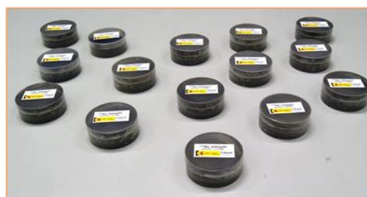
Figures 1 and 2 (above): Two sets of reference standards; one set from slag contaminated with Ra-226 and one set from cast steel contaminated with Co-60 (respectively)
