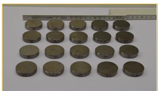
Figures 1 and 2 (above): Two sets of reference standards; one set from slag contaminated with Ra-226 and one set from cast steel contaminated with Co-60 (respectively)
