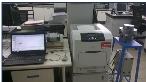
Figures 3 and 4: Testing of the CIEMAT and PTB Ge-based prototype spectrometric devices at end-user facilities in Portugal (Siderurgia Nacional) and Czech Republic (Vřtkovice Steel)
