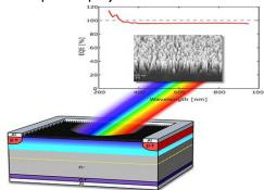
near unity (or near 100 %) quantum efficiency, meaning that they detect almost all the radiation present. A was black silicon induced junction photodiodes device was demonstrated with an external quantum efficiency above 96 % over the wavelength range 250–950 nm (see figure).
